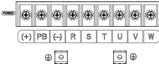
Figure 4-10 Main circuit terminals for the 7R5G/011P-015G/018P models
