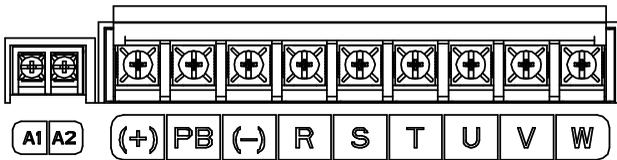
Figure 4-11 Main circuit terminals for the 018G/022P model
