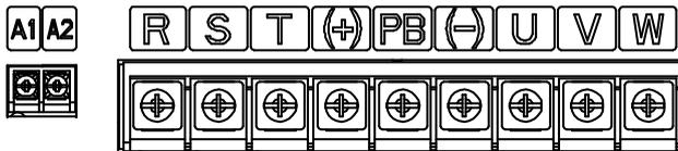
Figure 4-12 Main circuit terminals for the 022G/030P-030G/037P models
