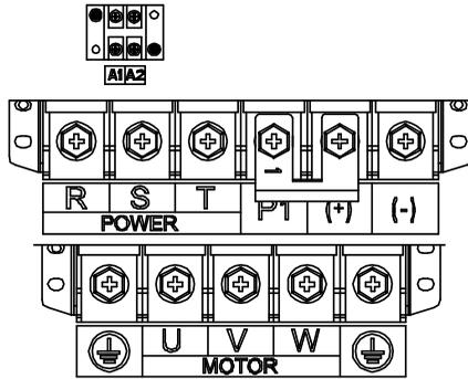
Figure 4-14 Main circuit terminals for the 075G/090P-110G/132P models
