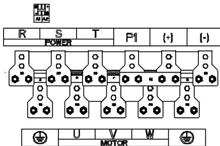
Figure 4-16 Main circuit terminals for the 220G/250P-315G/355P models
