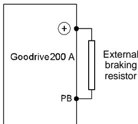
Installation of braking units:
