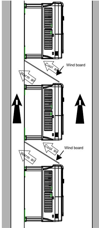
Figure 4-4 Vertical installation
