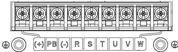
Figure 4-9 Main circuit terminals for the 0R7G-5R5G/7R5G models
