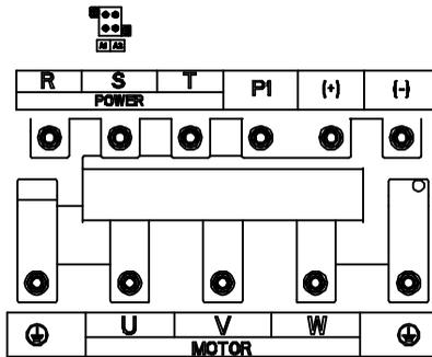
Figure 4-15 Main circuit terminals for the 132G/160P-200G/220P models
