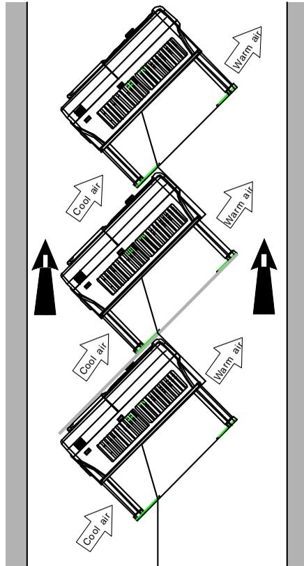
Figure 4-5 Tilt installation
