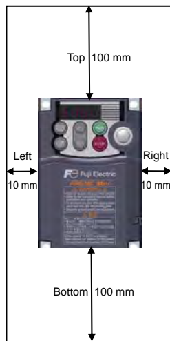
Figure 2.1 Mounting Direction and Required Clearances
